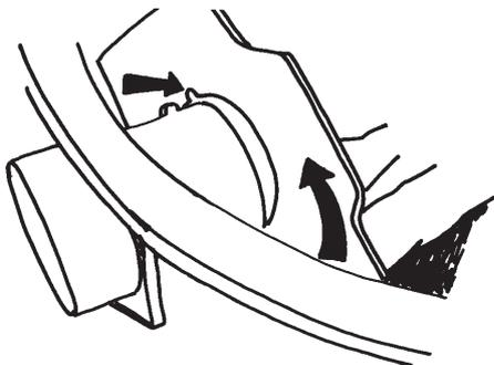
The opening in the card must line up and slide over the elevation on the inlet before you twist the cardboard stiffener to lock it.
