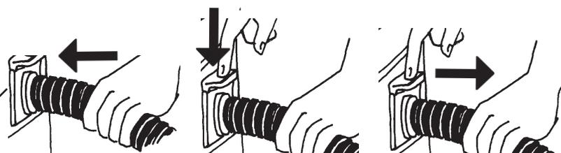
Push the hose in to the inlet at the cleaner until the hose locks. Press the button on the hose inlet downwards in order to remove the suction hose.
