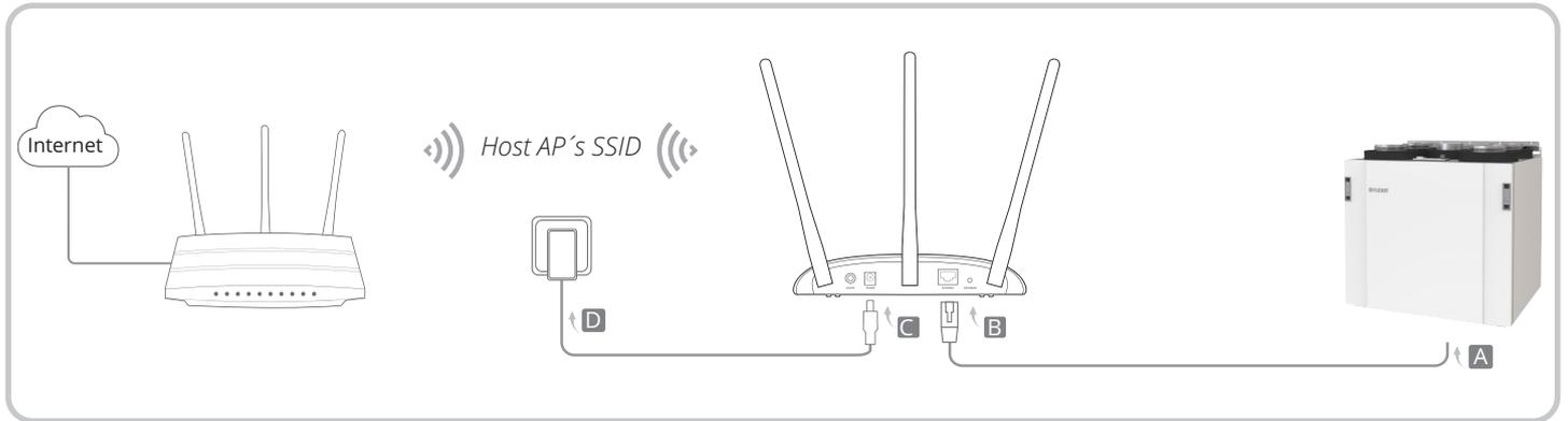
1. Connect the access point according to step A to D in the diagram.
