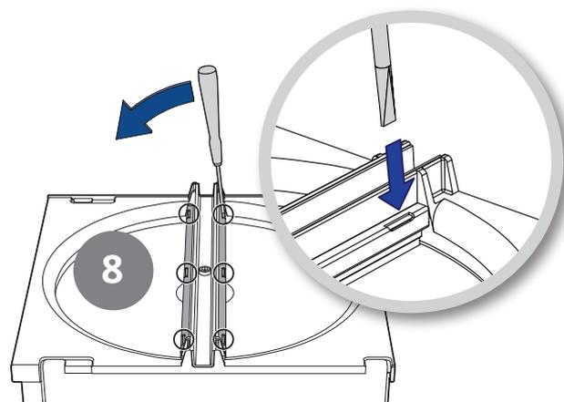
9. Pull the brush strips out of the groove.
