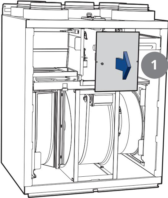
2. Disconnect the rotor's quick-release contact from the circuit board.
