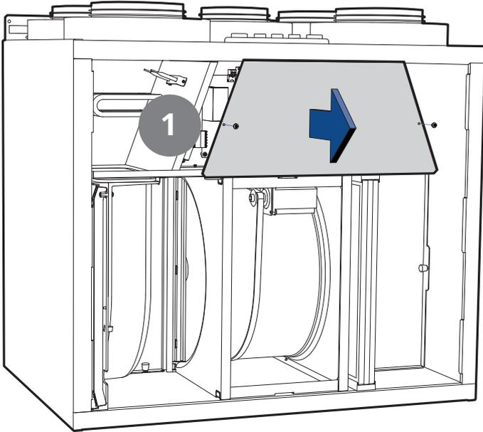
4. Pull the rotor module out about 2-3 cm.
