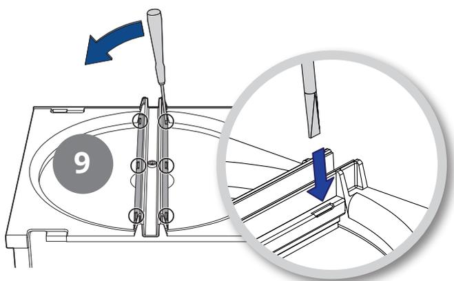
10. Pull the brush strips out of the groove.
