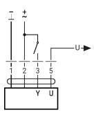
Override control and limiting with AC 24 V with rotary switch
