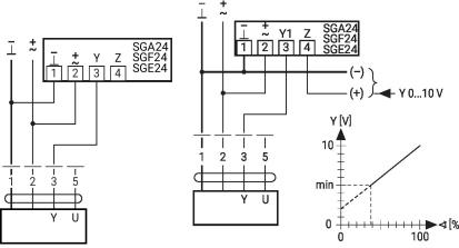
Control with 4...20 mA via external resistor
