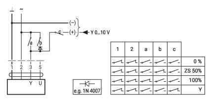
Control remotely 0...100% with positioner SG..
