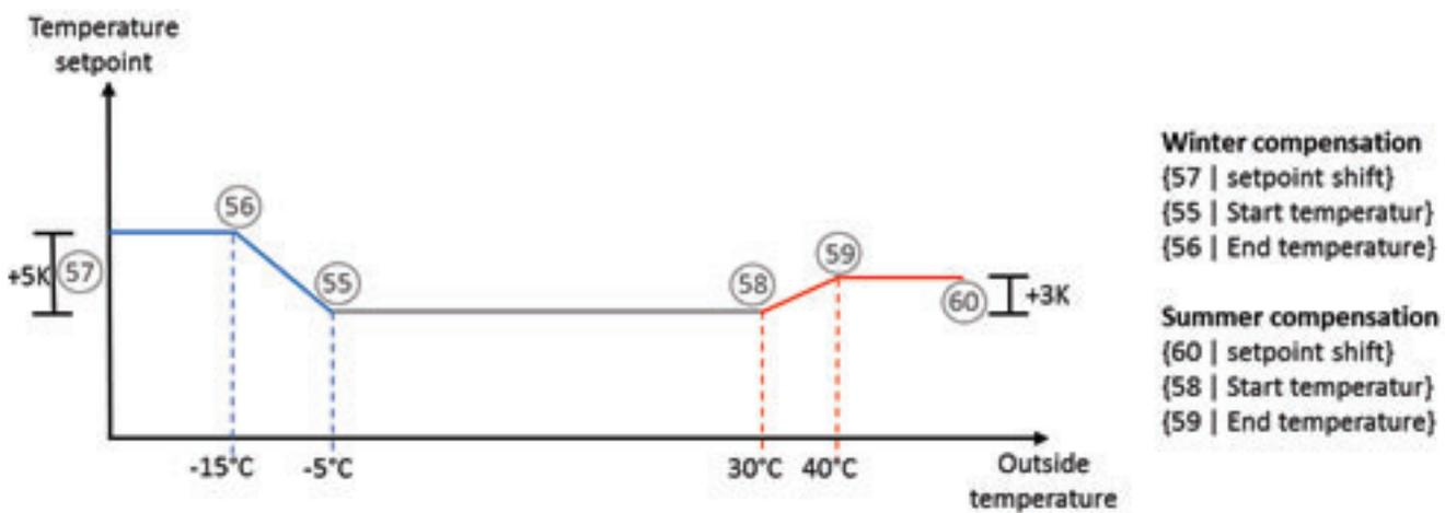
Outdoor temperature compensation is active when setpoint shift (57 or 60) is defined ( $\neq 0$ ) and the outside temperature is below/above set start limits (55 or 58). It has an influence on the temperature setpoint for both supply air and extract air cascade control.
