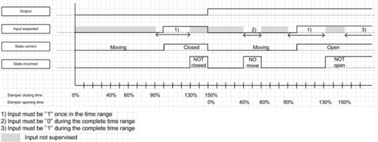
Incase fire dampers are equipped with own thermostat, during fire situation dampers close autonomously and feedback signal will become inactive and generate an A-alarm for fire situation with emergency shut-down.
