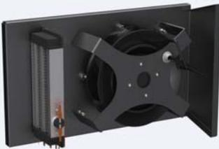
The Internal Pre-Heater Module is an essential accessory for NOTUS units operating in colder climates, especially in regions with prolonged subzero temperatures. It prevents frost buildup by warming incoming outdoor air before it reaches the heat exchanger. Equipped with a PTC heating element, the pre-heater ensures energy-efficient operation across various weather conditions.
