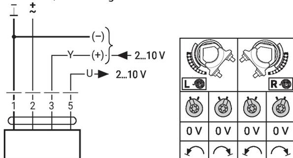
Wiring diagram piggy-back operation (mechanically coupled actuators)
