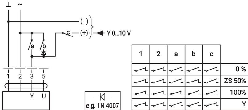
Control remotely 0...100% with positioner SG..
