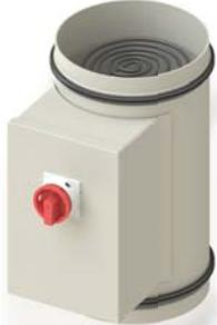
For subzero outside conditions, you should equip an electrical pre-heater to prevent ice forming inside the unit. This electrical pre-heater can connect to your BSK Heat Recovery Unit's fresh air intake vent.
