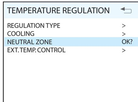
If supply air regulation is selected, no further settings can be set here. If extract air regulation is selected, the max. and min. supply air temperatures can also be specified.
