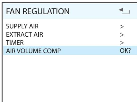
This dialog is identical for the supply air and extract air fans. The fans are adjusted individually to the desired capacity for the respective speed.
