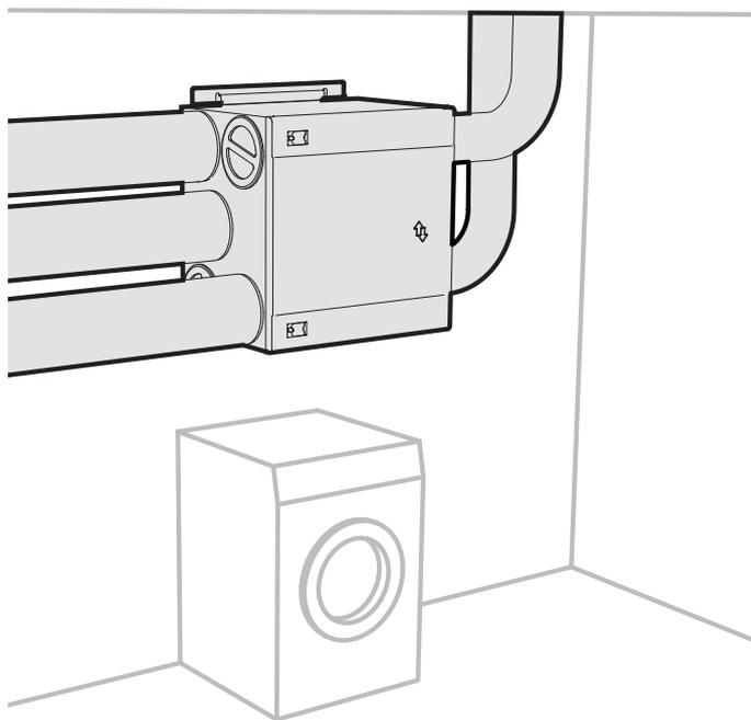
The attached wall bracket, as well as the enclosed bracket, are used for wall mounting. The same mounting is used whether the unit is installed with ducts up or out to the side (see Fig. 5). As standard, the unit has the mounting bracket mounted on the top. In case of sideways mounting, the rear wall of the unit must be dismantled, and then remounted after the mounting bracket has been moved (see Fig. 5 and "Chap. 2.3. Loft installation" on page 6).
