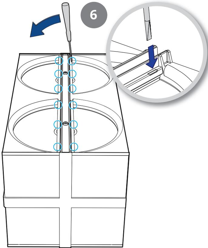
6. Pull the rotor module out and position it with the brush strip facing up.
