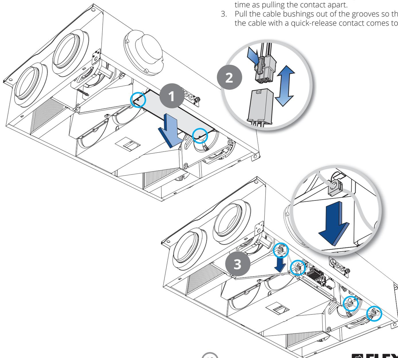
4. Undo the two screws securing the fan to the partition.
