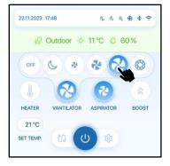
**Access Fan Speed Options:** Navigate to the home screen and tap either the VNT or ASP fan speed icon.
