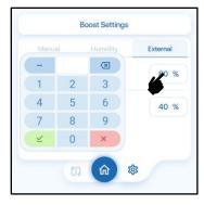
**Adjust Fan Speeds:** On the External Boost Settings page, customize the VNT and ASP fan speeds for when the device enters External Boost Mode.
