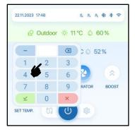
**Access Set Temperature:** Use the "SET TEMP." button to initiate the set temperature adjustment.
