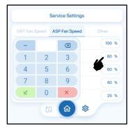
**Accessing ASP Fan Speed Settings:** In the Service Settings page, navigate to the ASP Fan Speed tab to modify the 5 preset fan speed values for the ventilator fan.
